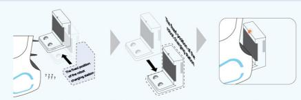
If the charging station has been moved away, you need to move the charging station back to its ancient position
