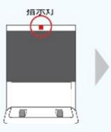
The charging indicator light shows red, indicating that the robot has successfully charged. Keep it all the time during starting the robot. The charging indicator light is always on.
