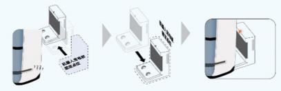
As shown in the figure, the fixed point of the charging pile is moved to the left, and the charging pile needs to be put back in place before the robot can charge normally.
