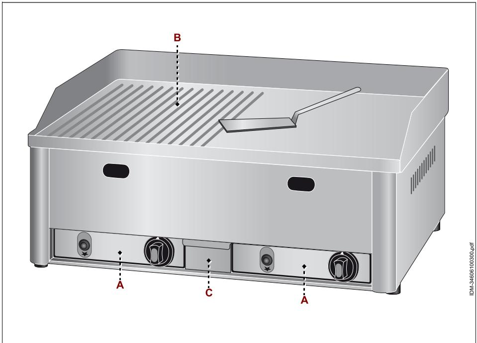
**A)** Control panel it is equipped with the control devices needed to operate the appliance (see "Control descriptions").
